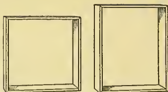
FIG. 128.—Comparison of tall and square sections of equal capacity.
