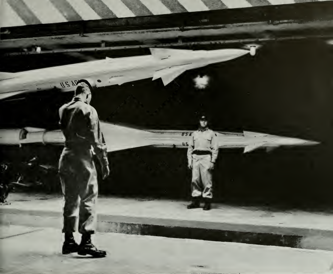
Ajax missile rises on elevator in underground storage area toward surface launching rack. Scene was at first operational NIKE installation in Maryland.
