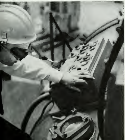
W. E. engineer checks white-hot batch of super-pure nickel in huge vacuum furnace.
