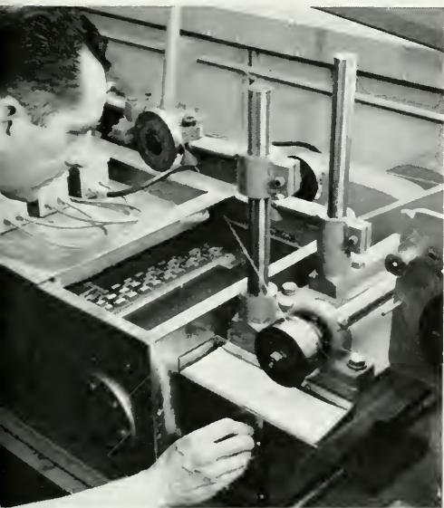
In new machine, wire enters drawing dies through an ultrasonically agitated liquid.
