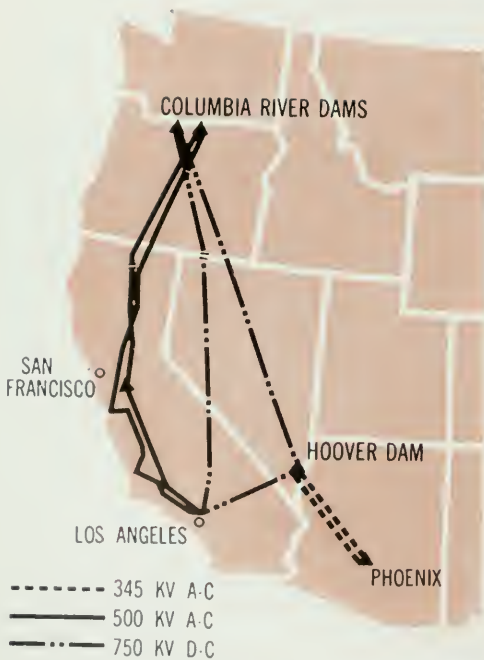
Pacific Northwest-Southwest Intertie: a vast power transmission network, now being built, which will interconnect 11 western states.
