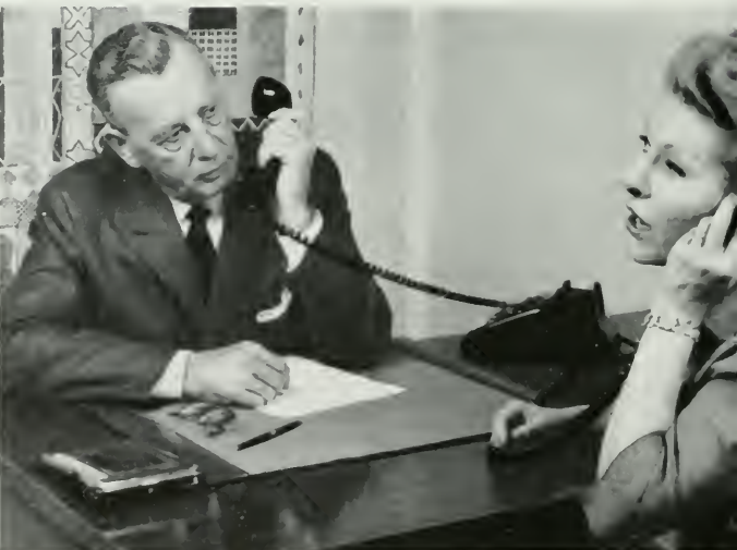
Watch case receiver enables third person to monitor telephone call and repeat incoming message so that a deaf person can lip read and still participate in the conversation.
