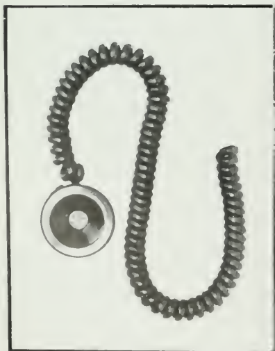
Watch case receiver enables third person to monitor telephone call and repeat incoming message so that a deaf person can lip read and still participate in the conversation.
