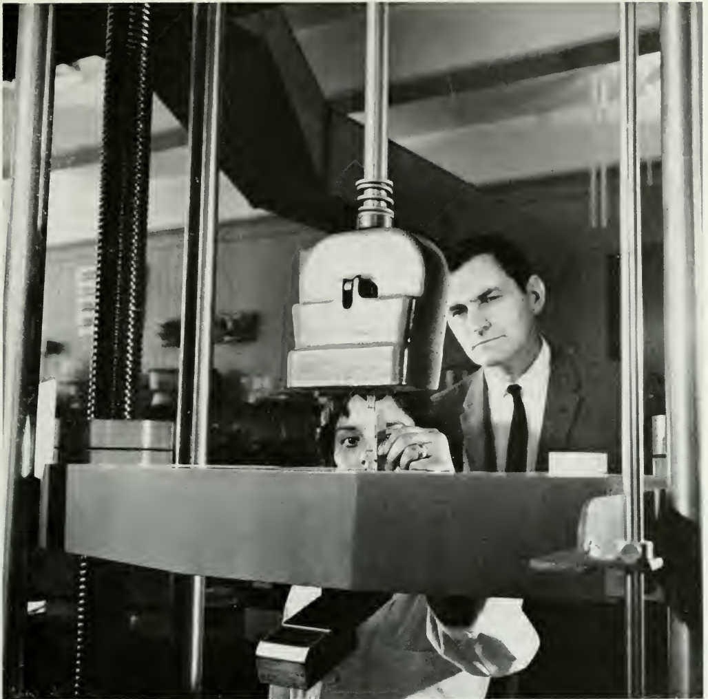
"This tensile test machine, capable of a 30,000-pound pull, is used to test tensile strength of plastic samples; this one being measured by Mrs. Shirley Stills is known as a polycarbonate."
