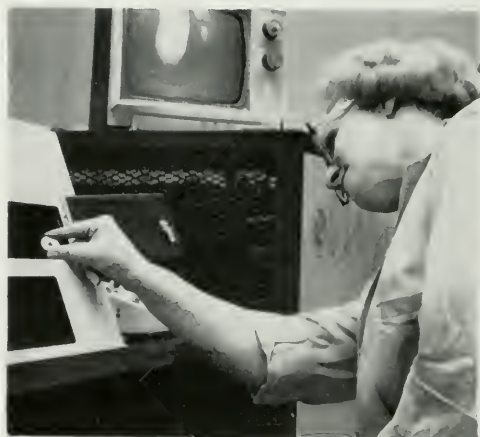
Die is put in oven for drilling by laser. Operator will watch by closed-circuit TV.
