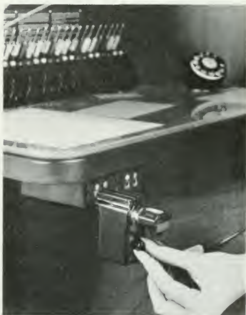
Small transistorized amplifier with volume control aids operator with hearing problem.
