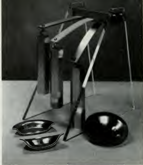
Left to right, strips of Bell Labs' new laminate, another laminate and steel weigh the same, support equal loads. Below, samples of new laminate that have been deep drawn.
