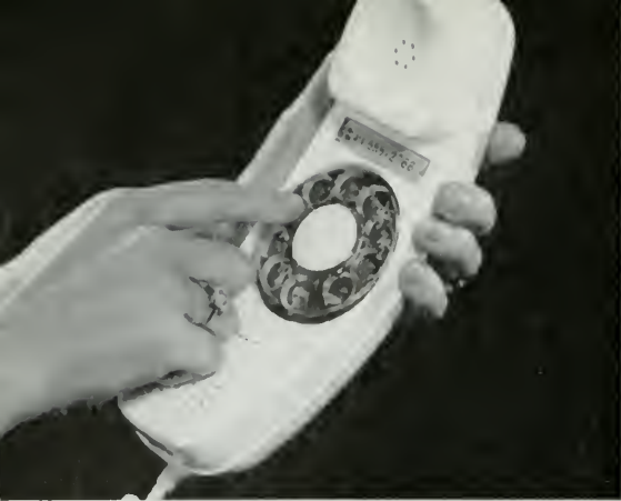
Light-weight Trimline phone has dial in handset, making dialing easier, more convenient.
