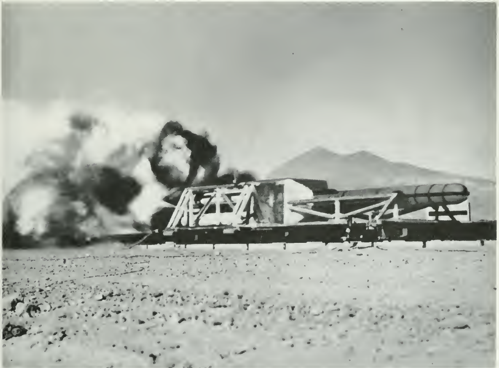
On Sandia's vast environmental test area, rocket-powered sleds shoot along 3000-foot sled track facility reaching velocities up to Mach 2.3 to simulate both launchings and impacts.
