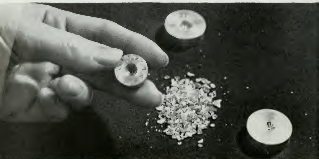
Diamond dies for drawing fine telephone wire are shown with loose industrial diamonds. Drilling diamonds for dies was a slow and laborious process before the application of the laser.
