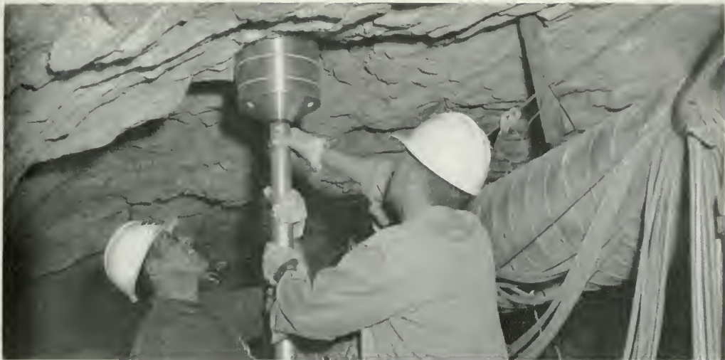
Sandia men install hydrodynamic gauge to measure nuclear explosion shock wave in Project Shoal experiment to improve ways of distinguishing earthquakes from underground explosions.
