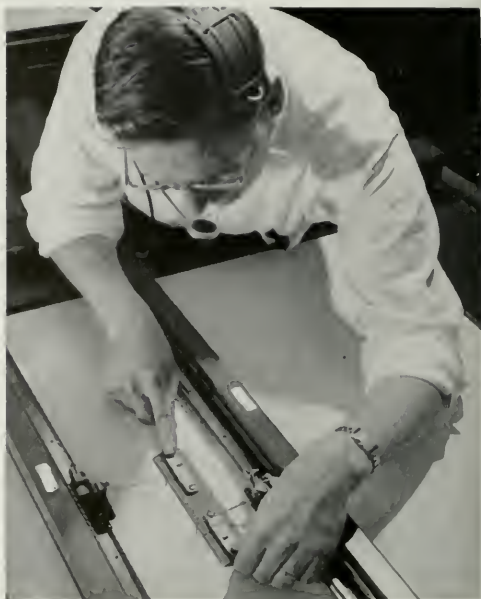
Bell Laboratories engineer sets up simulated firing course, during developmental stage of Nike, by plotting course of missile and target.
