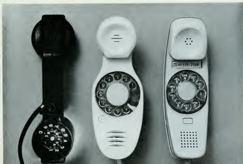
Three stages of the new phone's development show the telephone installer's test handset, the early "Schmoo" version with standard-size dial and the present-day Trimline handset.
