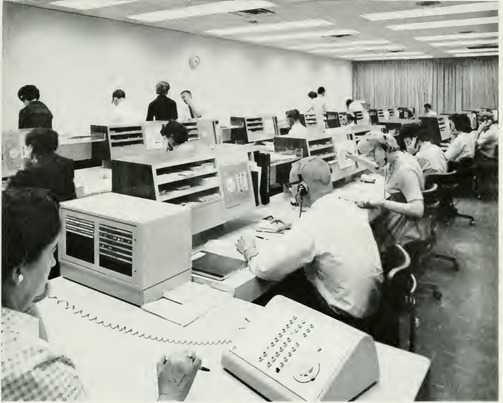
The Georgia Power Company's new customer service information center in Atlanta, Bell System's Model 2A call distributing system enables customer service representatives to handle up to 2,000 calls per day and provides for future expansion to 60 positions, 56 trunk lines.
