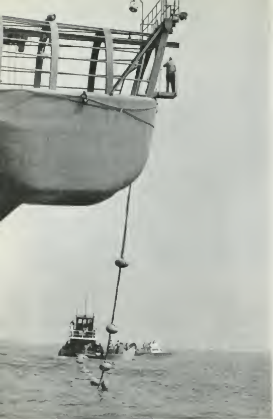
Shore end of transatlantic cable streams off distinctive bow of C. S. Long Lines.
