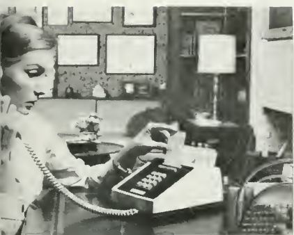
12-button card dialer as it would be used to "talk" to a bank's computer.
