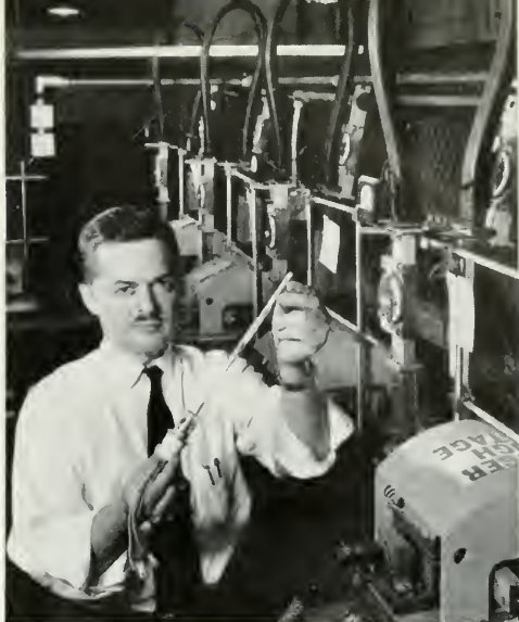
Traveling wave tube used in TH and TD-3 systems has a far greater power output than electron tubes used previously.
