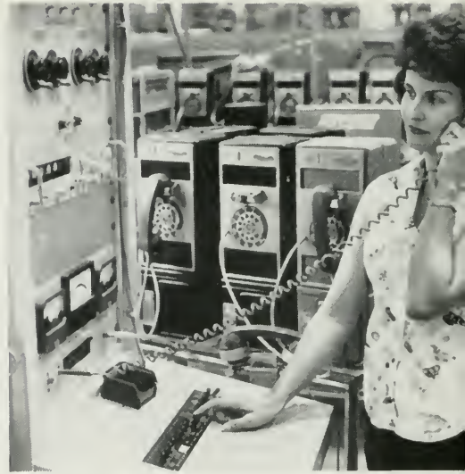
After final assembly, new coin telephones are individually tested on audio console.
