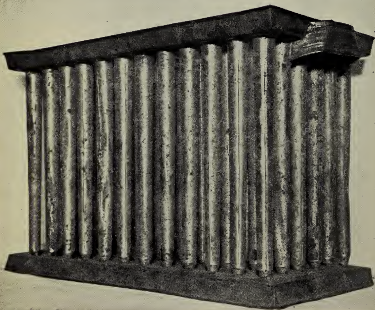
Upper—A fifteen tube candle mold and a hinged three-piece iron mold for twelve candles.
