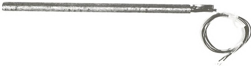
(b) STRESS GAGE SANDWICHED BETWEEN KAPTON LAYERS AND INSERTED IN PIPE
