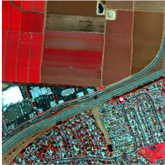
Figure 9. False color IR-R-G composite image of study area (healthy vegetation shown in red).
