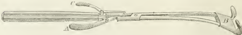
FIG. 5.—SOFT PALATE RETRACTOR.—A, lever to separate arms. B, the soft rubber band that closes the arms and holds the uvula out of the operator's way. C, the lever that raises the wedge. After the instrument is introduced behind the velum and the arms spread by the lever A, then the wedge retains them in position.
