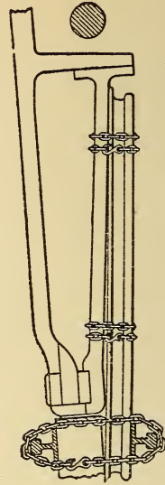
FIG. 33.—HOLDING UP REAR END OF ENGINE WITH RAILS CHAINED TO FRAME AND TENDER FOR BROKEN REAR DRIVING AXLE OR WHEEL.
