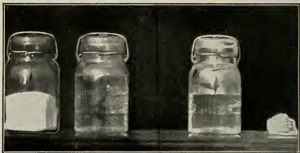
Figure 13—Materials for viscogen. At the left is sugar and water in which it is to be dissolved; at the right is lime and water in which it is to be dissolved
