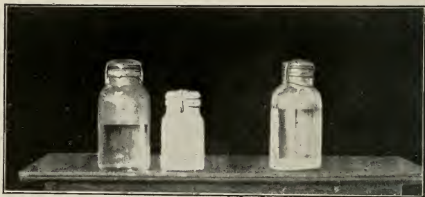
Figure 14—From left to right is sugar solution, slaked lime, viscogen. Note sediment of undissolved lime in bottle of viscogen at right
