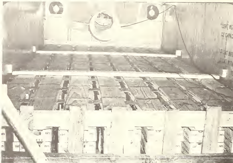
Figure 12. --Completed load of container "A" in express car. A 1- by 6-inch board covers the top of each row.
