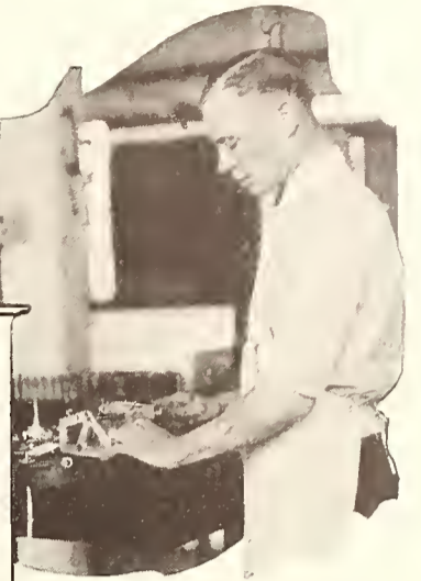
In assembling The Cheney motor the holes drilled and reamed in The Cheney motor frame become the bearing points for spindles and gears. The assembly of The Cheney motor is a very delicate and exacting operation.
