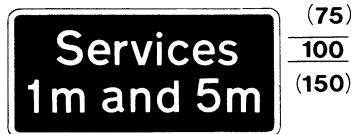
Distance to next two service areas Permitted variants: Second mileage may be omitted and the words "and information" may be substituted (See Directions 5 and 8) 838.2
