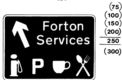
Direction to named service area at which fuel, parking, cafeteria and restaurant facilities are available Permitted variants: The name of the area may be varied having regard to the place where the sign is erected and that name may be omitted (See Directions 5 and 8) 838.1
