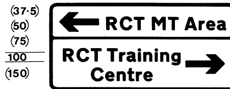
Direction to a Ministry of Defence establishment on a road extending from a junction ahead. 741.1
