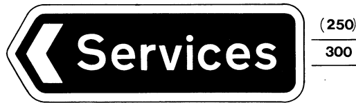
Direction to service area (See Direction 9) 916.1
