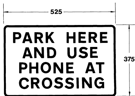
To indicate where large or slow vehicles should wait near an automatic railway level crossing within the meaning of Regulation 11(2) before the driver complies with Regulation 11(2)(b)
