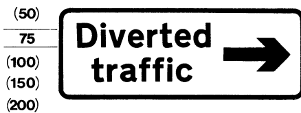
Temporary sign for diverted traffic from a junction ahead (See Direction 17) 755
