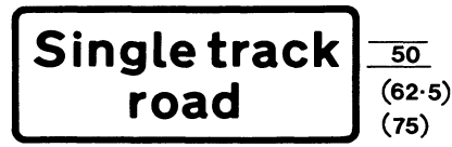
Road only wide enough for one line of vehicles Plate for use with signs in diagrams 516 and 517 (See Direction 12) 519
