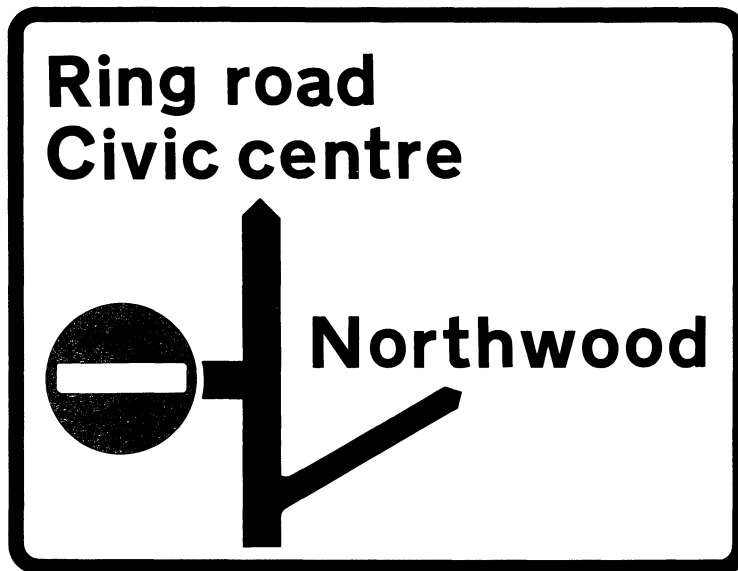
Same as 729 with variation for a road on which a prohibition exists Permitted variants: The No entry symbol may be replaced by a No right turn or No left turn symbol or a red bar as indicated by diagrams 816 and 817 where appropriate (See Direction 6)
