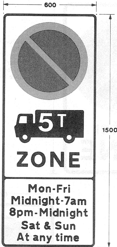
Entrance to a controlled parking zone applying to goods vehicles over 5 or 7.5 tonnes maximum gross weight Permitted variant: "7.5" may be substituted for "5" on the goods vehicle symbol (See Direction 6) 806.3
