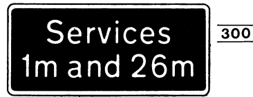
Distance to next two service areas (See Direction 9) 916
