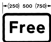
Plate for use with sign in diagram 801 Permitted variants: The legend may be varied to accord with any condition imposed on the use of the parking place without prejudice to Regulation 12(1)(g), or to "Viewpoint" or "Infor- mation". (See Direction 12) 805
