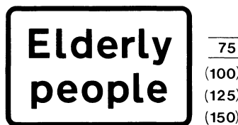
Plate for use with sign in diagram 544.2 Permitted variants: "Blind" or "Disabled" may be substituted for "Elderly" (See Direction 12) 547.4
