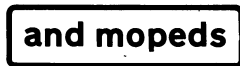
Plate for use with signs shown in diagrams 625 and 815 to indicate that mopeds may use the cycle track (See Direction 12) 625.2
