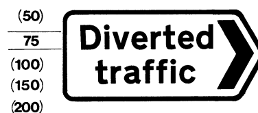
Temporary sign showing direction of route for diverted traffic (See Direction 17) 755.1
