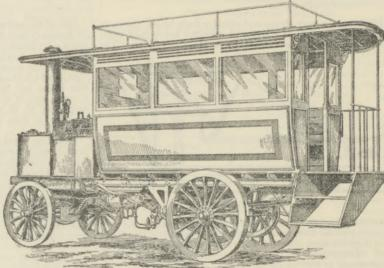
FIG. 23 -Thornycroft Steam Motor Omnibus.
