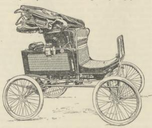
FIG. 7.-" Locomobile" Steam Carriage.
