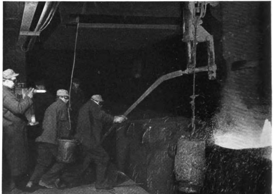
Air sampling at a steel pouring operation. A sample is being taken with an electrostatic precipitator and impinger in series by an industrial hygiene engineer from the USPHS. The sodium fluoride in double sealed cellophane bags is thrown into the mold during the pouring of the steel.
