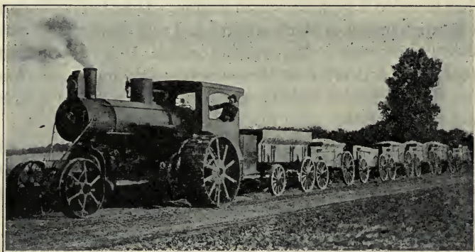
Fig. 251. An undermounted double-cylinder steam tractor.
