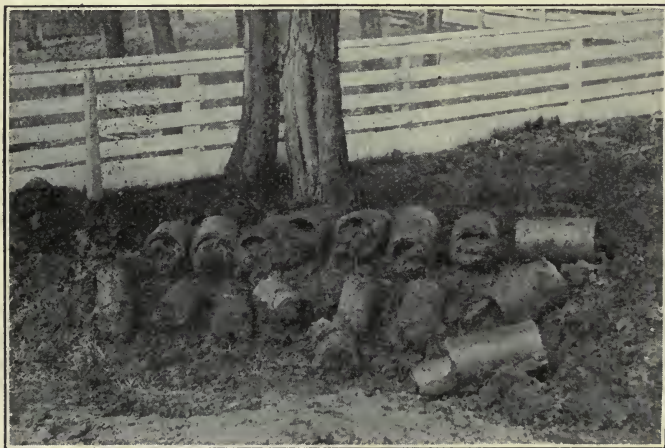
Fig. 65. A tile drain which became completely obstructed by roots from a willow tree.
