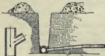
Fig. 60. Sketches showing proper method of joining lateral drains to mains. From Ohio Exten. Bul. 47.
