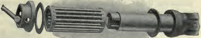
Fig. 103. A roller bearing for wagons. The hub of the wheel fits over the rollers shown.
