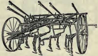
Fig. 149. A two-row cultivator with straddle seat placed well to the rear. The gangs are guided by a treadle device.
