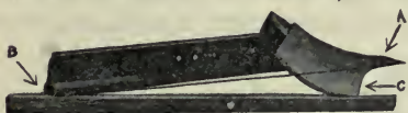
Fig. 111. A share with the proper form at the wing. The contact of "bearing" at C should be about 1\frac{1}{4} inches wide for a 16-inch plow.
