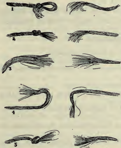
Fig. 155. The ends of bands which have not been made into perfect knots. (After Steward in Trans. Am. Soc. A. E.)
