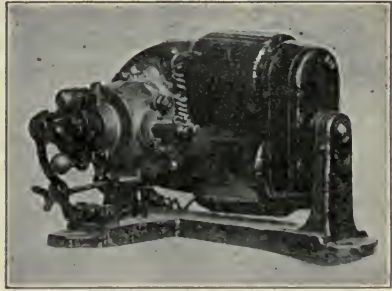
Fig. 232. A dynamo called the Auto-sparker.
