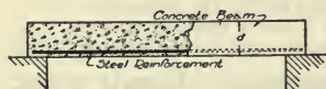
Fig. 262. Sketch showing the proper location of steel in a concrete slab to resist tensile stresses due to bending.
