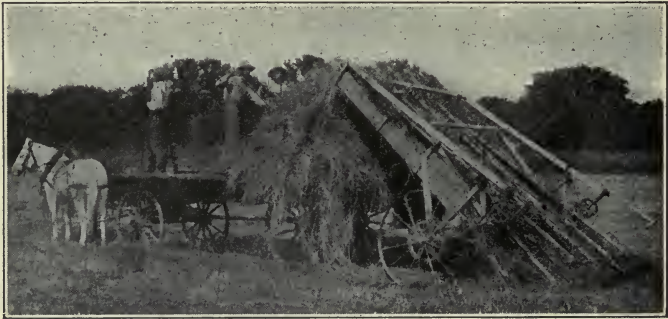
Fig. 167. A fork hay loader at work.
