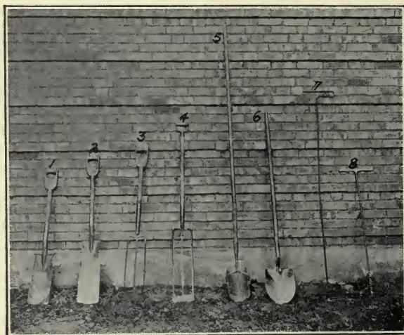
Fig. 53. Hand tools used in digging tile ditches. Nos. 1 and 2 are square-end tiling spades, 3 and 4 are open or skeleton tile spades, 5 is a tile scoop or crumber, 6 is a round-point shovel, 7 is a tile hook, and 8 a soil auger.
