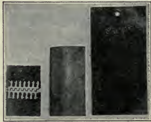
Fig. 200. Sample of canvas, rubber, and leather belting.
