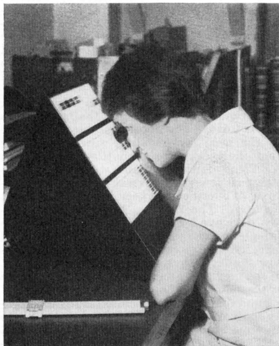
Figure 2.—Examining the fine lines of a spectrogram (the picture taken with a spectrograph) as a means of detecting the trace elements present in foods. The quantities are so small that they had been completely overlooked in other methods of analysis.
