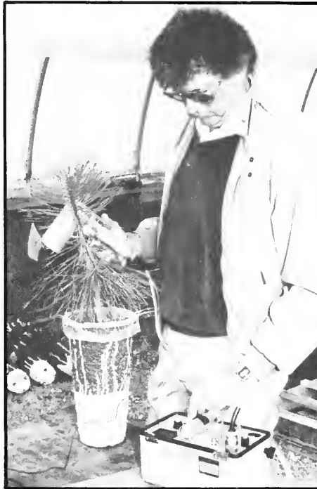
Plant Physiologist Pat Heidmann uses a diffusion porometer to measure moisture stress of a ponderosa pine seedling.
