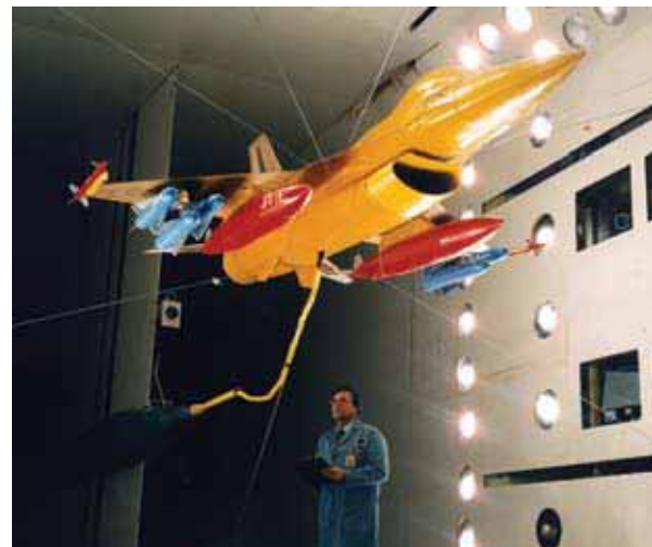
Jerome T. Foughner with F-16 model in Transonic Dynamics Tunnel during flutter tests with external stores.
