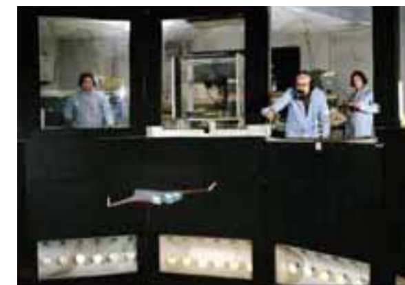
Free-spinning tests of a Blended Wing Body model in the Langley 20-Foot Vertical Spin Tunnel.
