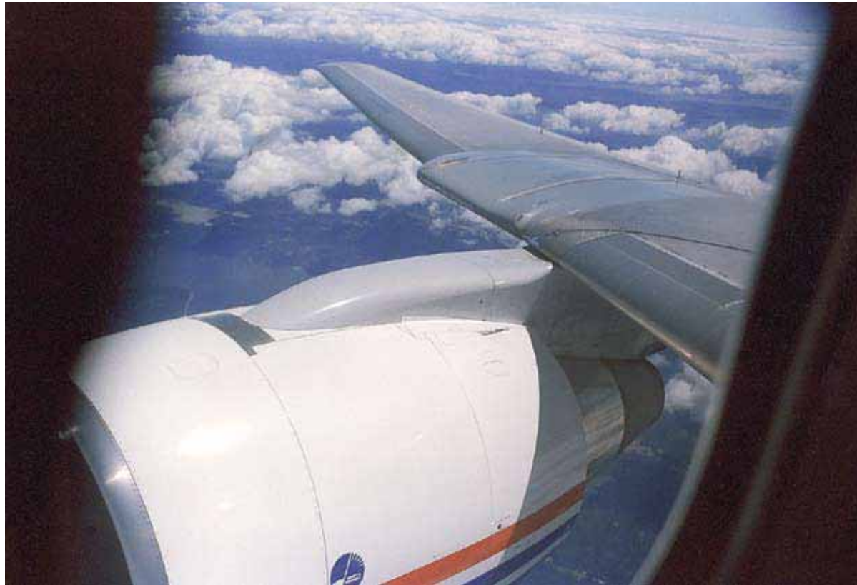
In-flight view of the natural laminar flow glove mounted on the Boeing 757's right wing during boundary-layer noise sensitivity evaluations.
