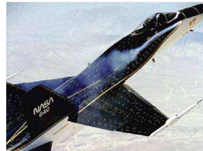
NASA's F/A-18 High Angle of Attack Research Vehicle uses smoke injected into vortex flow to illustrate vortex breakdown position for angles of attack of 20 degrees (top) and 30 degrees (bottom).
