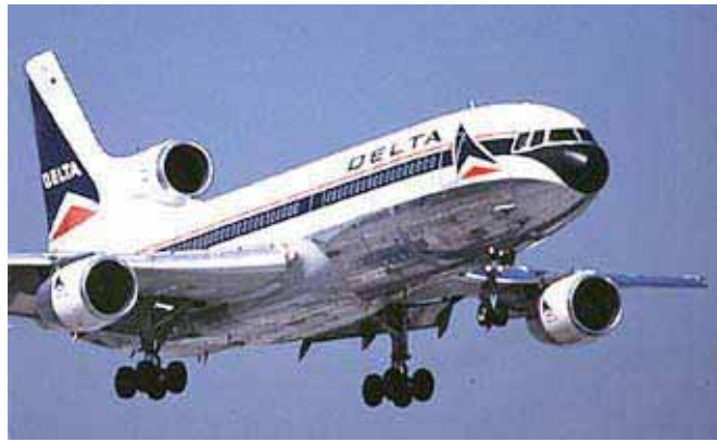
The Lockheed L-1011-500 was the first commercial transport to use active load control.
