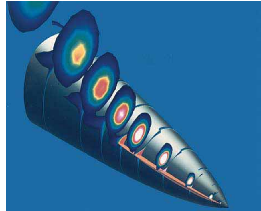
Computational results of the effect of forebody strake deflection on the F/A-18 forebody.
