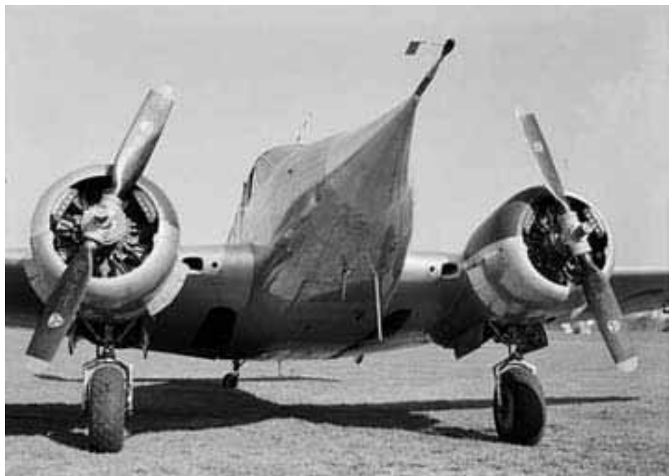
Nose boom with angle of attack vane on C-45 transport used for gust alleviation research.
