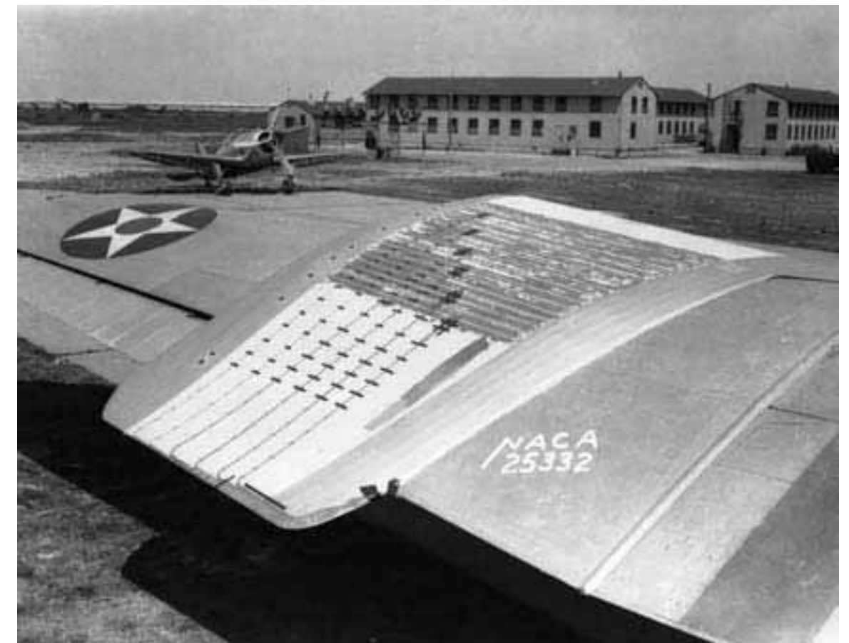
B-18 wing glove tests conducted by NACA (top) and close-up view of the glove panel used in natural transition studies (bottom).
