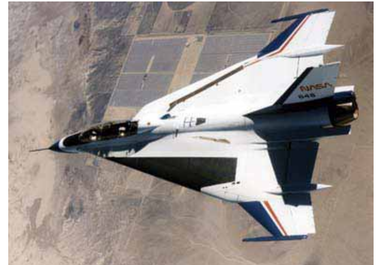
Modified F-16XL Ship 2 with supersonic lamina-flow glove installed in left wing panel.
