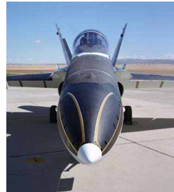
Close-up view of the forebody strakes on the F/A-18 High Angle-of-Attack Research Vehicle research airplane.
