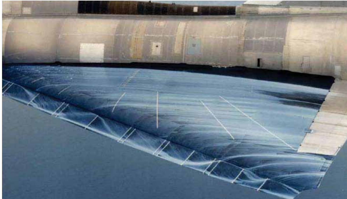
Surface-oil studies illustrate multiple vortex flows seen on the leading edge.
