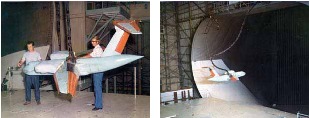
Technicians David R. Brooks and Benjamin J. Schlichenmayer prepare a free-flight model of a USB transport for tests in the Full-Scale Tunnel.
