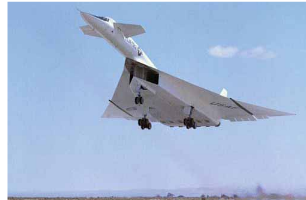
The XB-70 bomber, designed for supersonic cruise at Mach 3.0.
