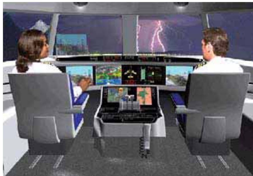
Artist's concept of advanced cockpit display with synthetic vision head-down and head-up displays.
