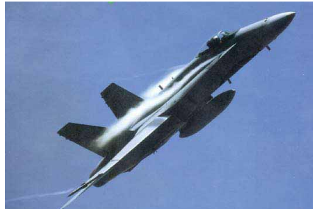
Strong vortical flow emanating from the wing-body strake of the F/A-18 is clearly defined by natural condensation in air.
