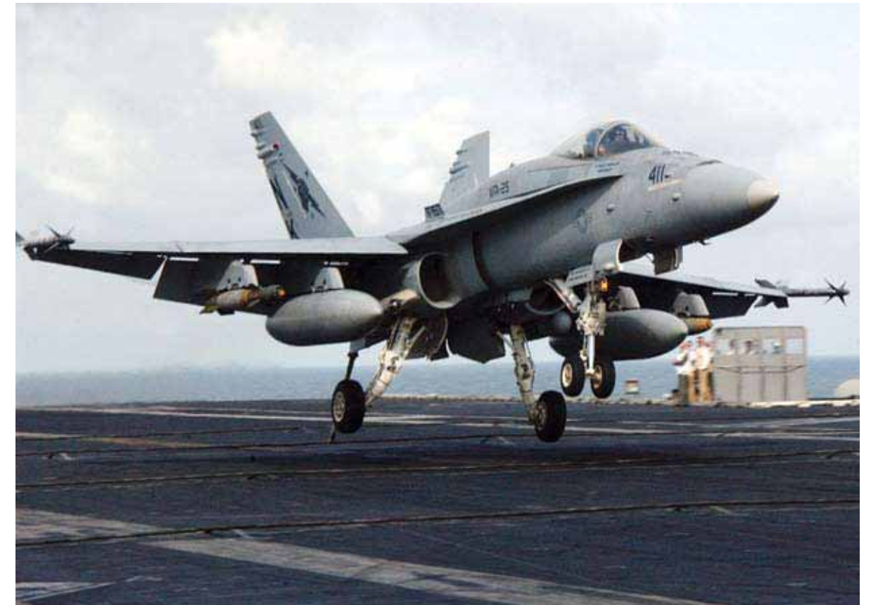
McDonnell Douglas successfully developed and applied an active control system to suppress wing/store limit cycle oscillations in production F/A-18 aircraft
