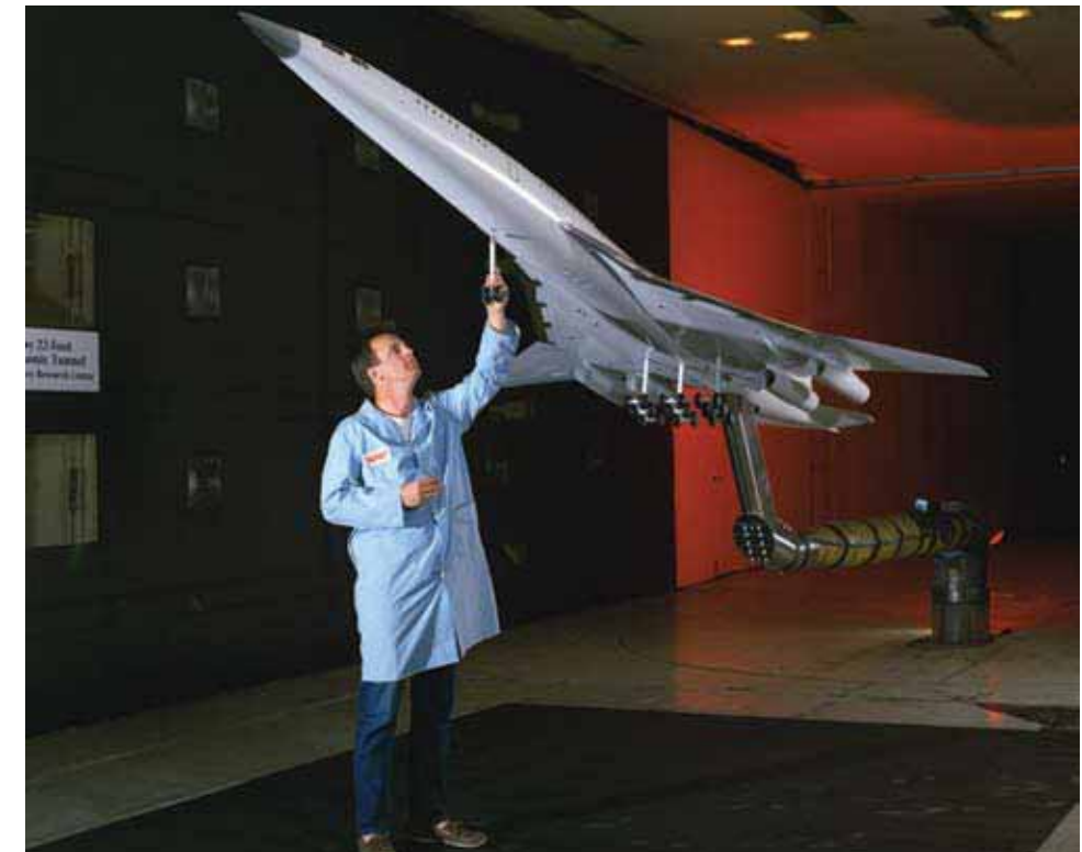
Technician Michael E. Ramsey inspects a 19-ft long model of the High-Speed Civil Transport Reference H configuration during tests of takeoff and landing characteristics in Langley's 14- by 22-Foot Subsonic Tunnel.
