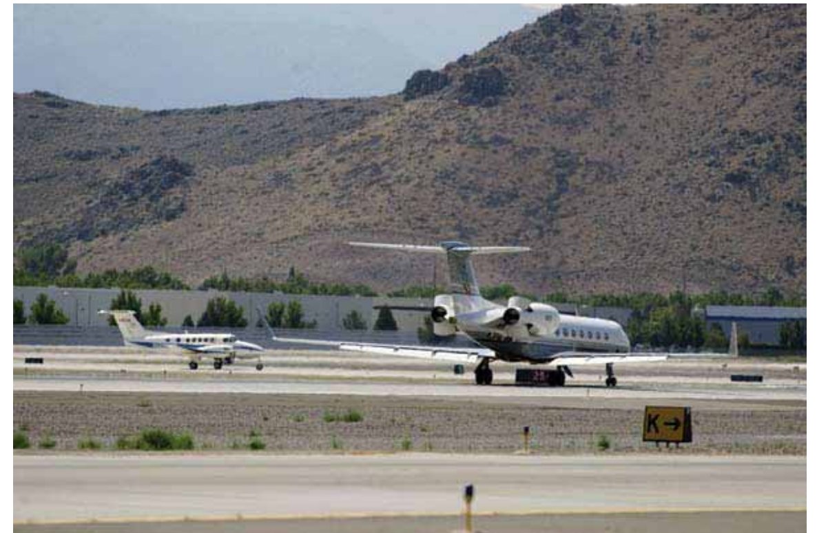
Simulated runway incursion by NASA King Air airplane (left) during Reno evaluations of incursion prevention systems on Gulfstream V airplane (right). Note the deployed engine thrust reverser doors on the Gulfstream V as the pilot takes corrective actions to avoid the potential collision.
