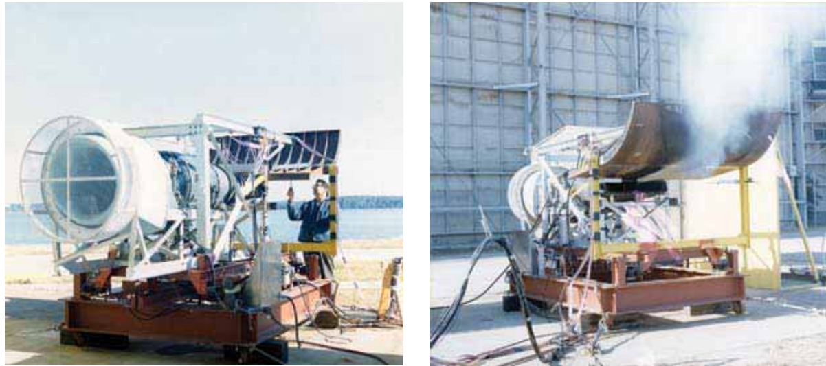
Engine test-stand investigation in preparation for tunnel tests of modified Aero Commander airplane. Photo on right shows turning of flow around upper surface blown flap.
