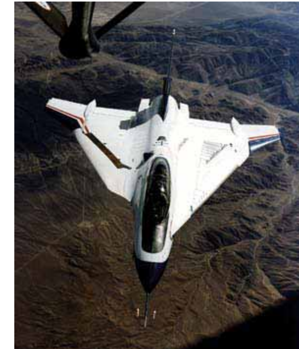
NASA's F-16XL was modified with an active suction laminar flow glove on its left wing for exploratory assessments of supersonic laminar flow control.
