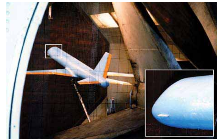
Model configuration tested in Strake Technology Research Application to Transport Aircraft project.
