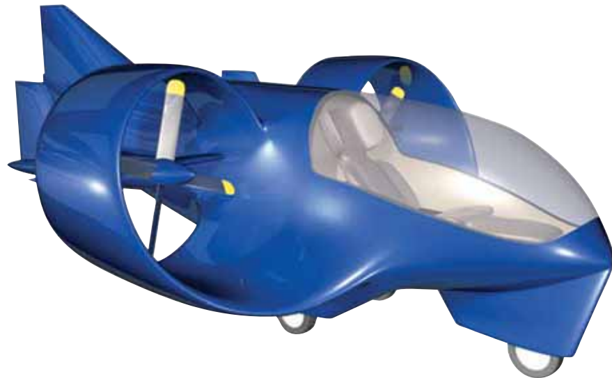
Notional Spiral Duct Personal Air Vehicle.
