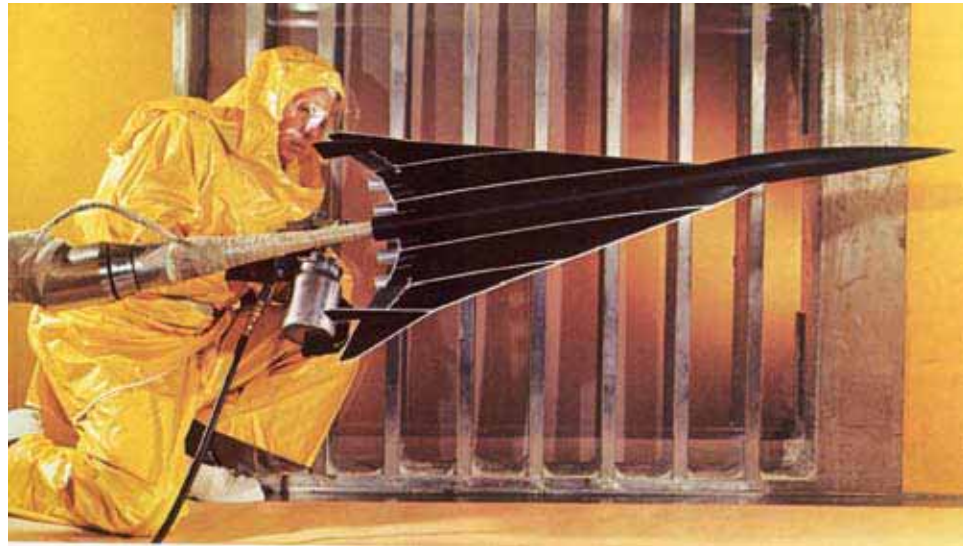
SCAT-15F model being prepared for flow visualization tests in the Langley Unitary Plan Wind Tunnel.
