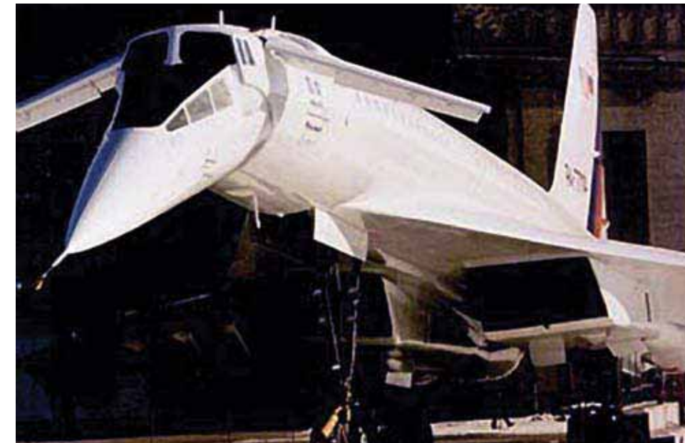
The Tu-144 supersonic transport used a variable-geometry drooped nose for improved visibility during low-speed operations.
