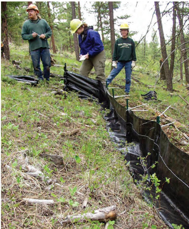
Example of a sediment fence used to measure postburn hillslope erosion.
