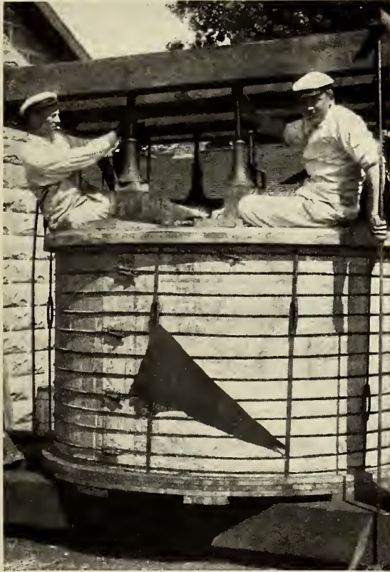
THE SPECIAL HOOP AND PRESS USED TO FORCE THE WATER FROM THE CHEESE.
