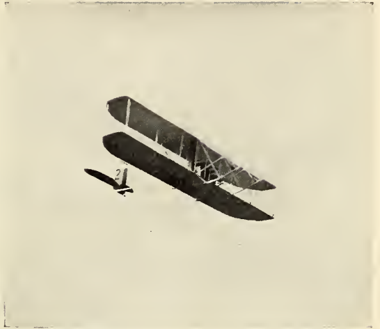
A WRIGHT BIPLANE IN FLIGHT (NEW TYPE). Showing the vertical and horizontal rudder in the rear.
