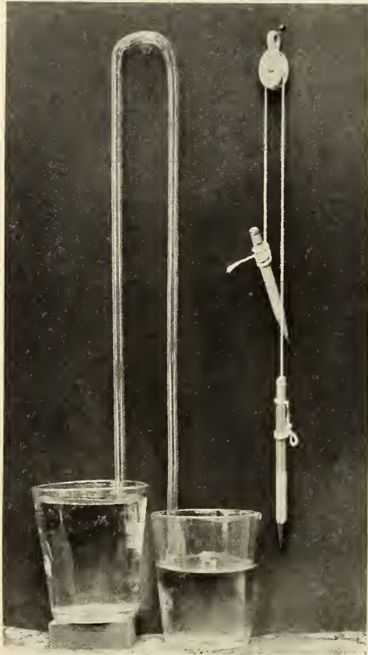
THE LONGER AND HEAVIER COLUMN OF WATER IS "PULLING" UP THE SHORTER COLUMN AS THE HEAVIER LEAD-PENCIL IS PULLING UP THE SHORTER PENCIL.
