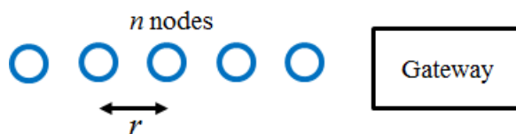
Figure 12. A simple network of n nodes and one gateway each separated by a distance r .
