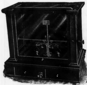
No. 98 ASSAY BALANCE (NEW) 5-Inch Beam. Sensibility, \frac{1}{100} Milligramm
