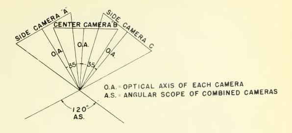
Figure I-B. Horizontal view of arrangement of plate holders and lenses in a multiple-lens camera. E and D cameras are arranged in the same relative positions to the "B" camera as A and C cameras, but they have fore and aft positions respectively.
