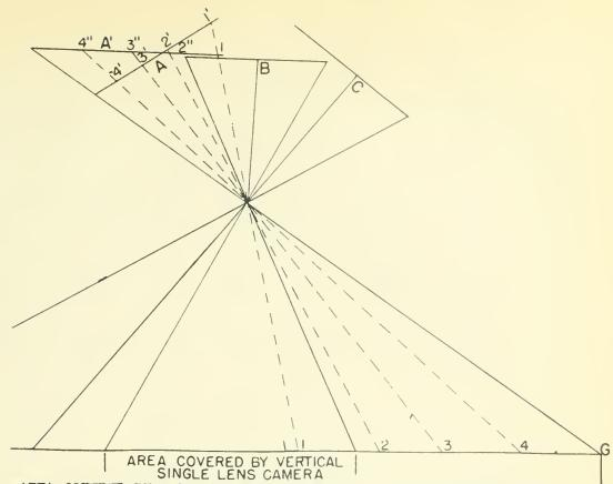
AREA COVERED BY A MULTIPLE LENS CAMERA. PROPORTIONAL AREAS ALSO COVERED IN REAR AND FORWARD DIRECTIONS BY D & E LENS.
