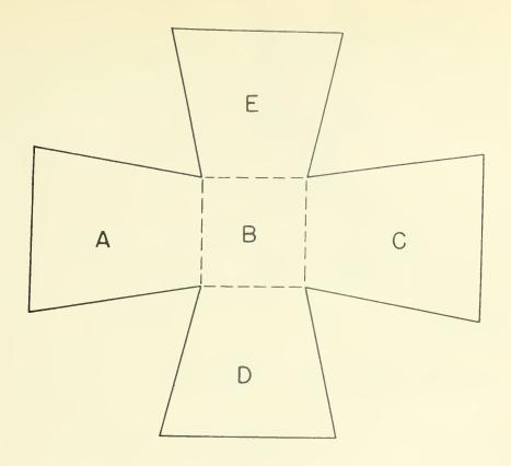
Figure II-B. Outline of ground area covered, and shape of transformed photographs taken with multiple-lens and single-lens cameras.
