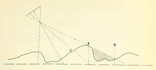
Figure IV. The effect of topography on the displacement of images on oblique photographs.
