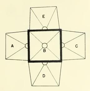
Figure I-A. Vertical view of arrangement of camera compartments in a multiple lens camera:
