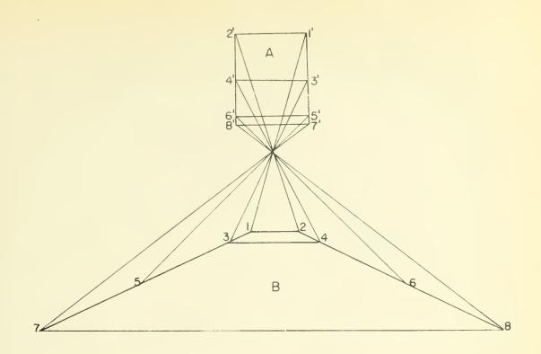
Figure III. Relation of the image lines, on an oblique negative, of lines on the ground parallel to the horizontal axis of the oblique negative. "B" outlines the ground area reflected on an oblique negative.
