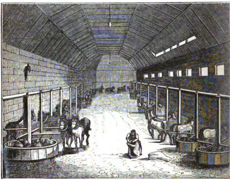
Fig. 1270. represents the rude grinding apparatus used at the lavaderos , or gold washings, in Chile. The streamlet of water conveyed to the hut of the gold washer, is received upon
