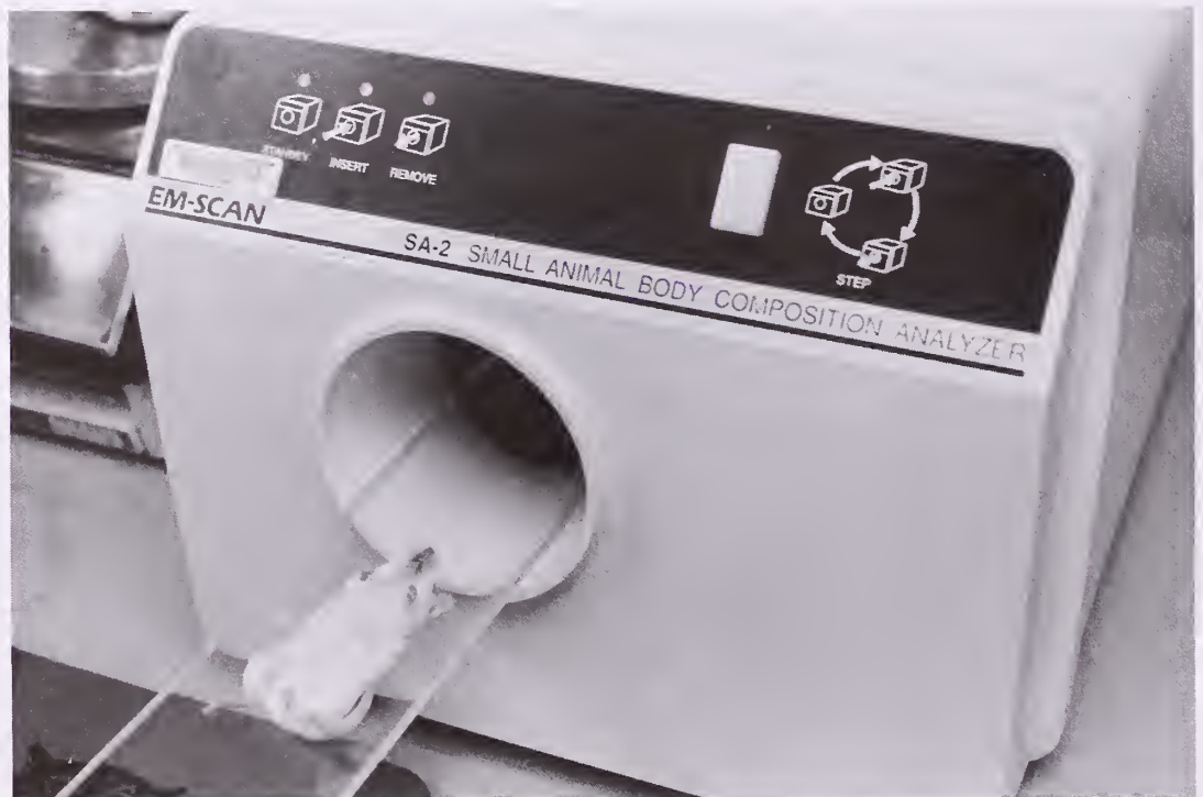
Figure 1. An anesthetized mouse is inserted into the TOBEC instrument for measurement of electrical conductivity subsequently used to predict fat-free mass.
