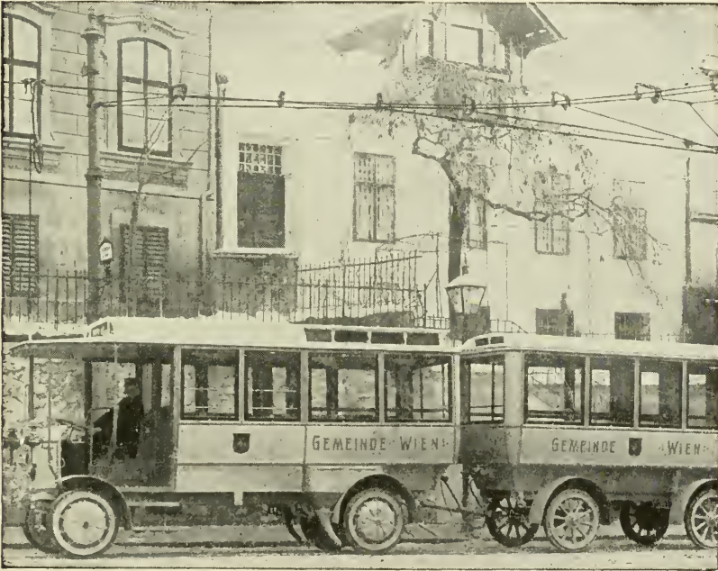
Fig. 9. Four-Motored Vienna Trackless Trolley with Trailer
