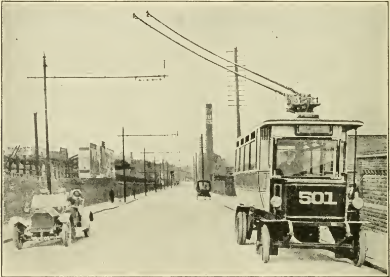
Fig. 17. View Showing How Trackless Trolley Can Draw Up to the Curb
