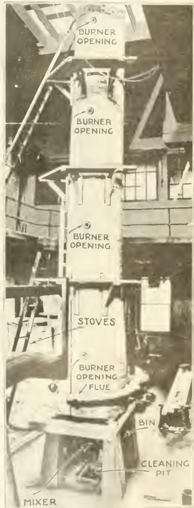
FIG. 1. 30-FT BRICK COMBUSTION CHAMBER ERRECTED IN THE CASE LABORATORY
