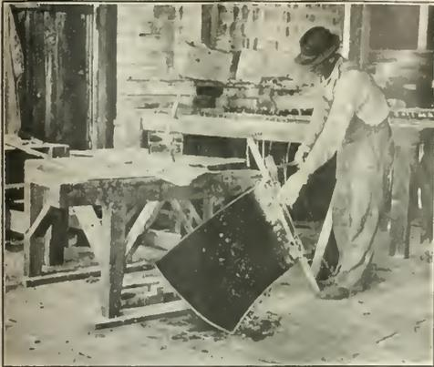
CUTTING OUT CONDUCTOR BARS FROM SPENT ANODES
