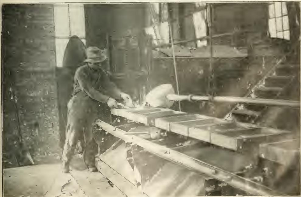
POURING ZINC INTO MOLDS AND SKIMMING
