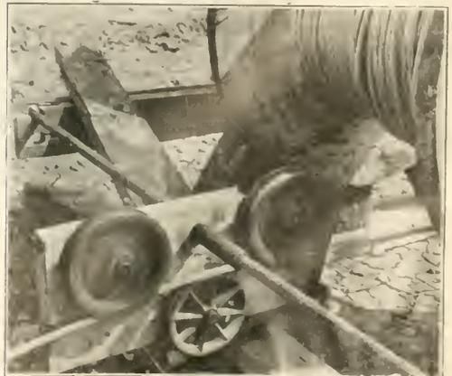
METHOD OF STRAIGHTENING WIRE ROPE BY MEANS OF THREE PULLEYS
