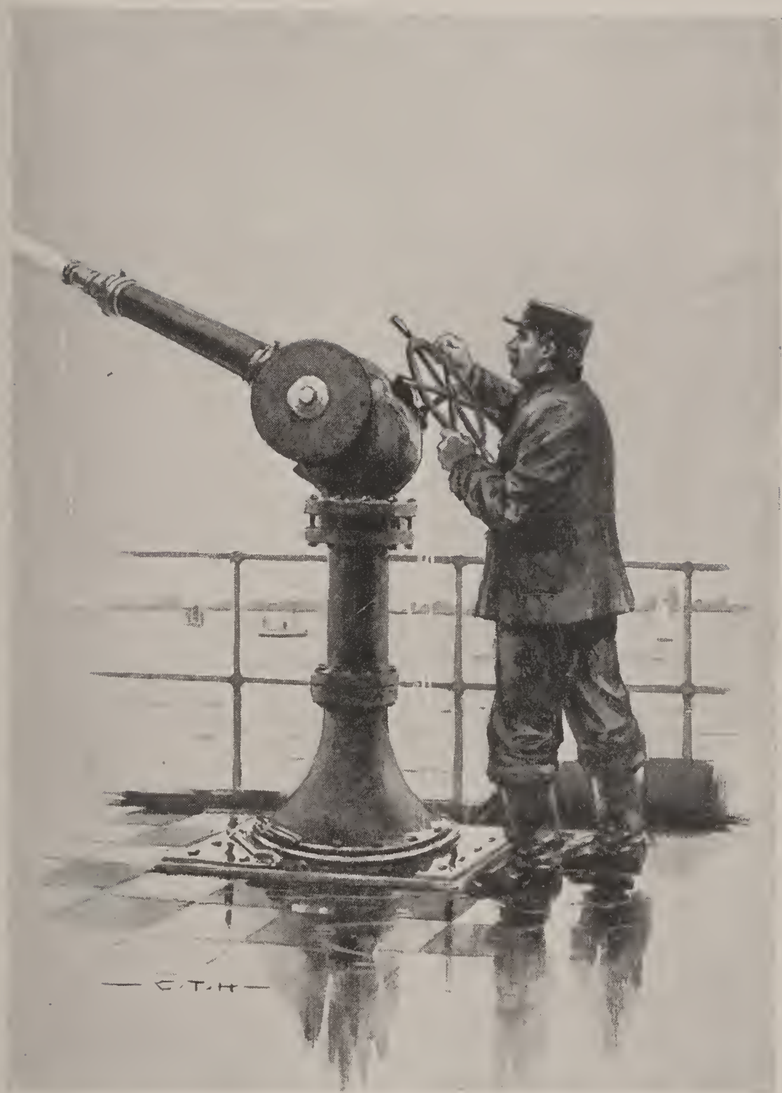
GIANT MONITOR-NOZLE ON THE FIRE-BOAT "NEW YORKER."
