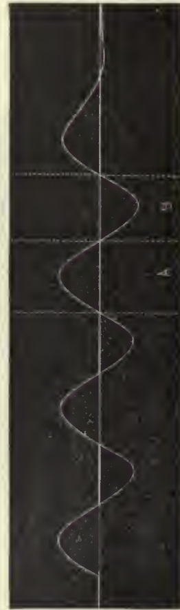
Fig. 3. Graphic representation of the sinusoidal current obtained from magneto electric apparatus employed by the author since 1883.
