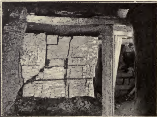
FIG. 110.—Undercut coal, fallen in blocks.
