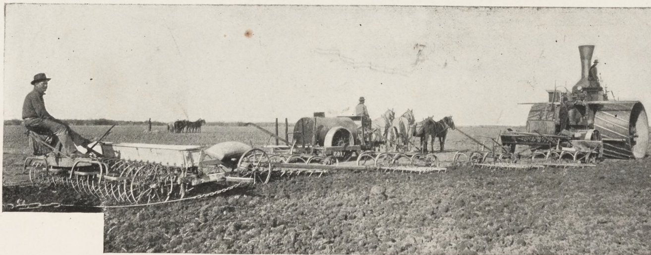
110 Horse-power Traction Engine Plowing, Harrowing, and Seeding, at one operation, 50 acres a day
