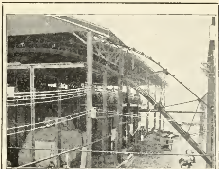
Jeffrey Conveyor handling Bagasse from mill storage floor and boiler house, at the Sugar Refinery of Fajardo Sugar Company, Fajardo, Porto Rico.
