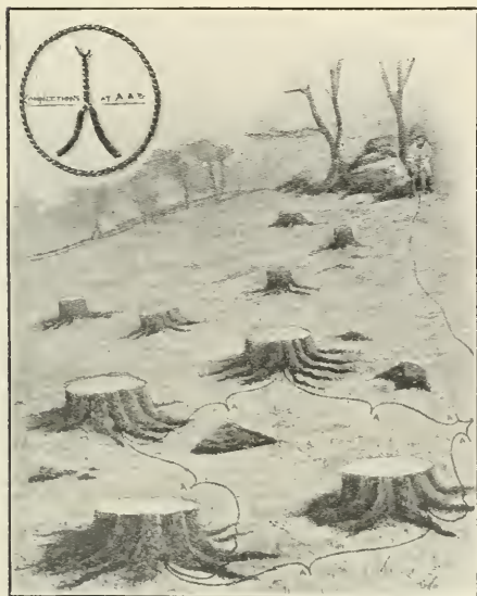
Plan of wire connections for exploding dynamite in the removal of stumps.
