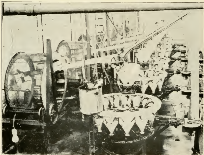
Can-filling machines. These automatic machines are great labor-saving devices, filling the cans with fruit or vegetables direct from the cooker
