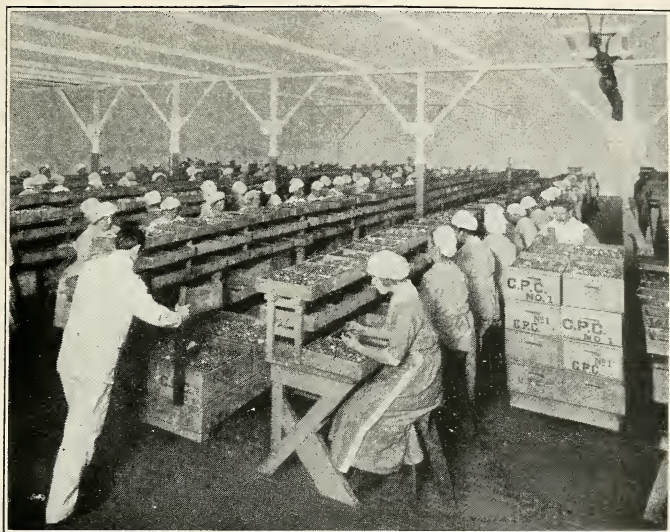
Taking care of a surplus product. Assorting and stemming a big shipment of cherries in a canning plant
