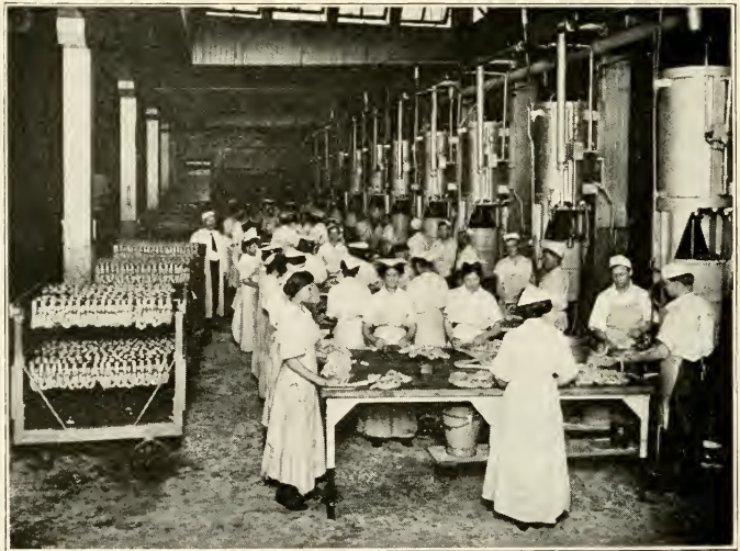
In a sausage factory. Here pork that has been changed into sausage is now being stuffed into "casings" and made ready for marketing
