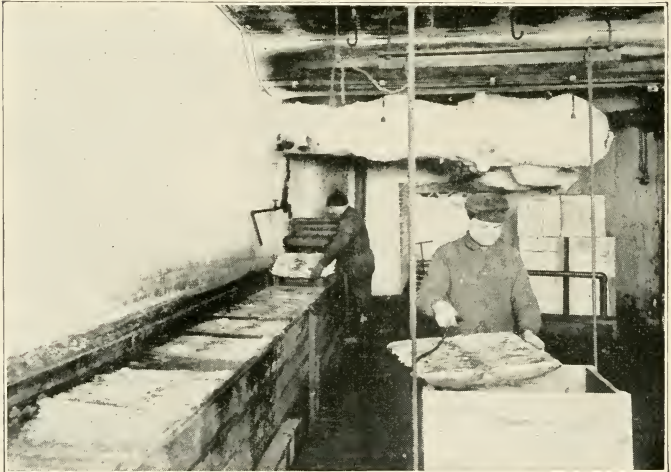
Glazing small frozen fish in tanks in the freezing room of a wholesale fish market. The thin ice which forms on the fish when dipped in water makes their preservation still surer
