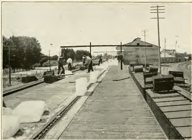
Icing a "passenger express refrigerator" car with an automatic chain ice conveyor
