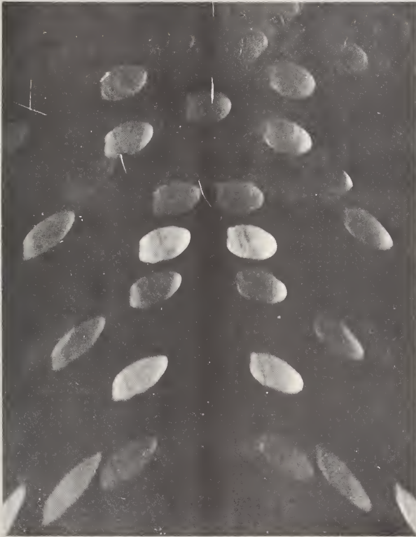
Fig. 2. Diffraction pattern of a ruby rod in which each spot is a crude topograph.
