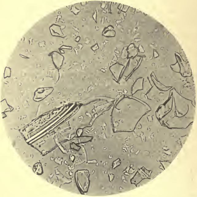
Fig. 42.—Photomicrograph of prepared chalk from one of the common tooth-powders. Imagine brushing the teeth (and gums) with such a brush as that pictured in Figs. 40 and 41, and with this sharp, gritty material on it. Not only would it damage the gum and cause retraction, but it would wear away grooves in the root of the tooth after it is exposed. Most other powders and pastes that are effective "cleansers" contain similar gritty material. This is the chief cause of "erosion."
