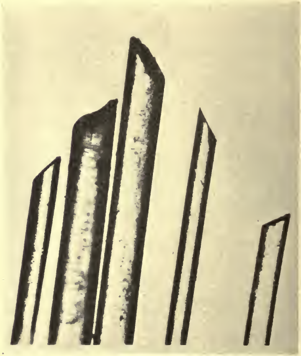
Fig. 41.—Photomicrograph of bristles taken from the tooth-brush shown in Fig. 40. Could it be possible to brush the teeth (and gums) with such an instrument without damage to the gums?
