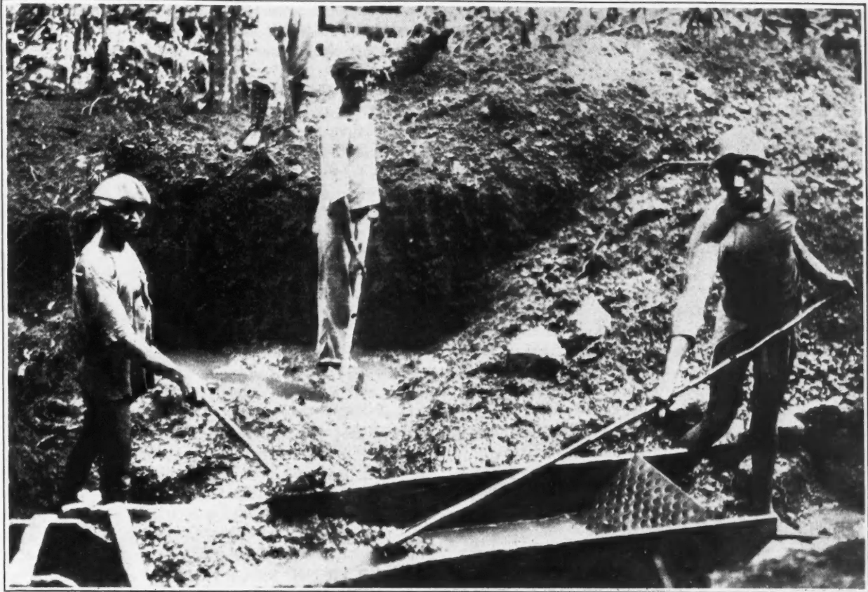
Testing placer ground by crude hand washing
