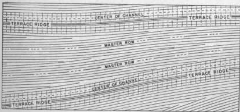
FIGURE 36.—Arranging point rows between master rows on terraced land places all the rows more nearly on the contour than does any of the methods shown in figure 35. This is the most intricate of the four suggested arrangements.
