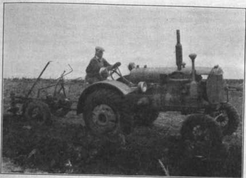
FIGURE 22.—The rotary-type terracer developed by the Agricultural Engineering Department of Iowa State College.
