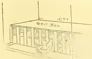
Fig. 2.—Swinging trough for bones and grit. Size, three feet by ten feet, and four inches deep at bottom below slats.
