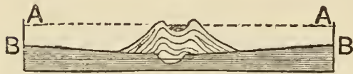
FIG. 52.—Embankment of a river. BB, original slope of valley. The light shading shows successive layers of deposit; AA, level of river.
