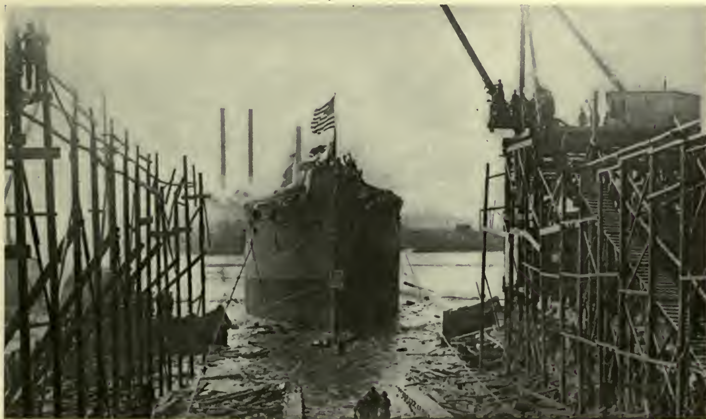
Fig. 66. Coyote, Wooden Ship Built by the Foundation Company. She Is 281 Ft. Long and Is the First of a Big Fleet Building at This Company's Plant on the Passaic River
