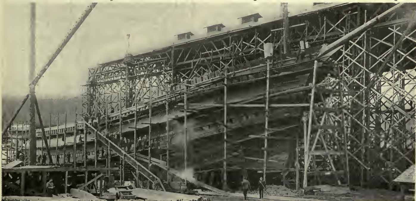
Fig. 91. A 255-Foot Auxiliary Schooner, From Designs by Tams, Lemoine & Crane. Planked Ready For Shutter
