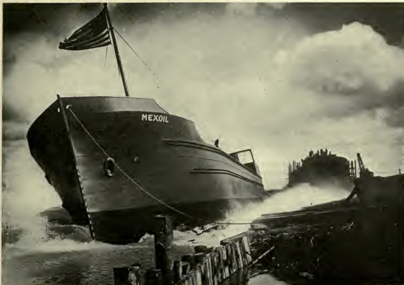
Fig. 69. Launch of the Mexoil, a 3,000-Ton Vessel, Built by the Alabama-New Orleans Transportation Company at Violet, La., For the Mexican Petroleum Company
