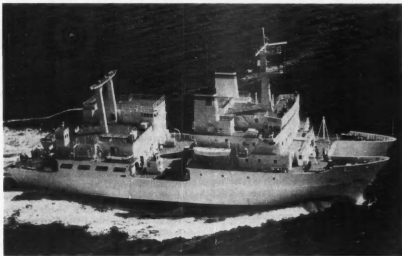
THE CATAMARAN. Labeled an "Innovation for Oceanology," the USNS Hayes is the first departure from conventional hull designs in the U.S. Navy's oceanographic ship construction program. The dual-hulled, 246-foot-long ship will be a major facility for underwater acoustics and oceanographic research. The ship is operated by civil service crews of the Military Sealift Command. In addition to the regular 44-man crew, it carries 30 Naval Research Laboratory scientists and technicians aboard when conducting experiments at sea. (Official U.S. Navy Photo)
