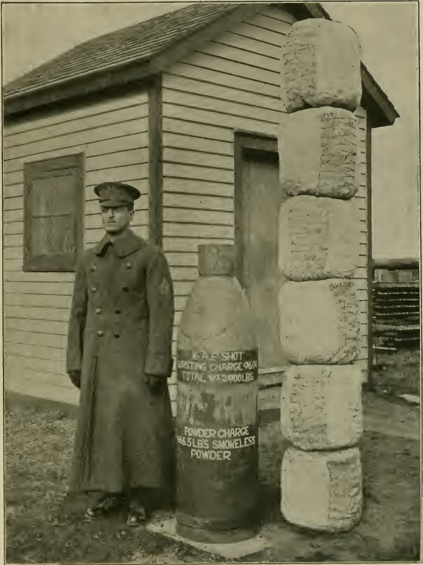
FIG. 61. Projectile and Powder Charge for American 16-inch Gun ; Weight of Charge, 666.5 lb. nitro-cellulose powder
