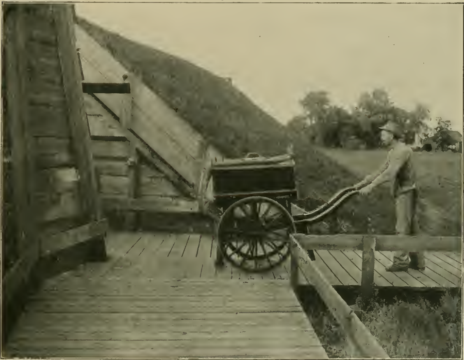
FIG. 48. Truck for Conveyance of Liquid Nitro-glycerine, Repauno, U.S.A. (By permission of E. J. du Pont de Nemours Co.)
