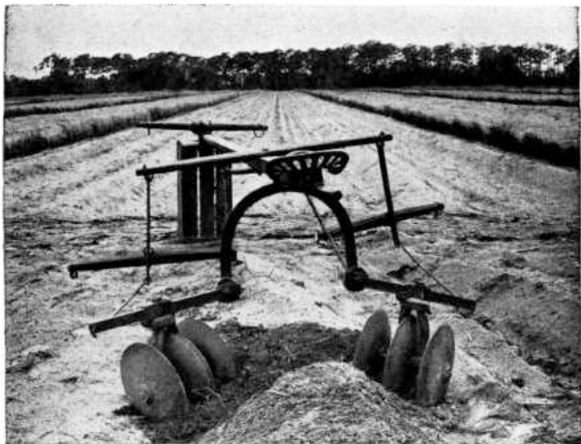
Figure 3. —A type of asparagus ridger used to a considerable extent in some asparagus-growing sections for renewing the ridges.
