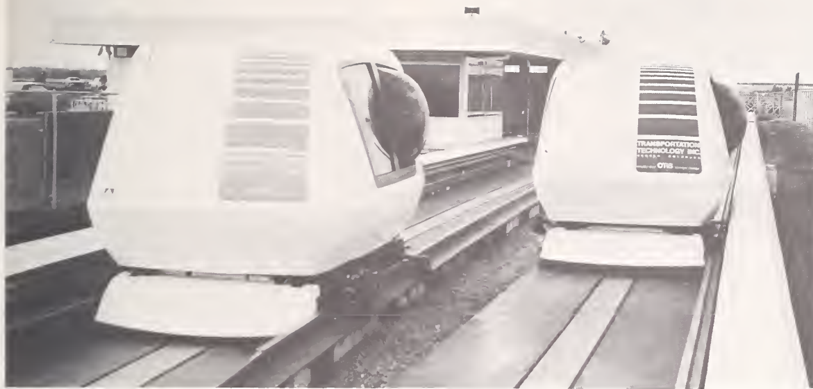
The Transportation Technology Air Cushion Vehicle was first demonstrated at Transpo 72 and then was evaluated in extended use at Dulles Airport outside Washington, D.C.
