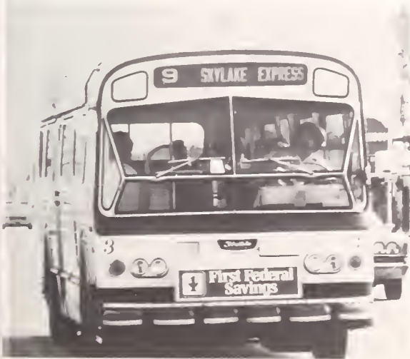
A bus with a signal preemption device (above destination sign) provides express service along the I-95/Northwest 7th Avenue corridor in Miami.
