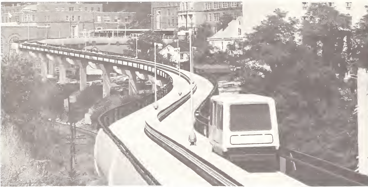
The Morgantown PRT system links distant reaches of the West Virginia University campus by elevated automated guideways.
