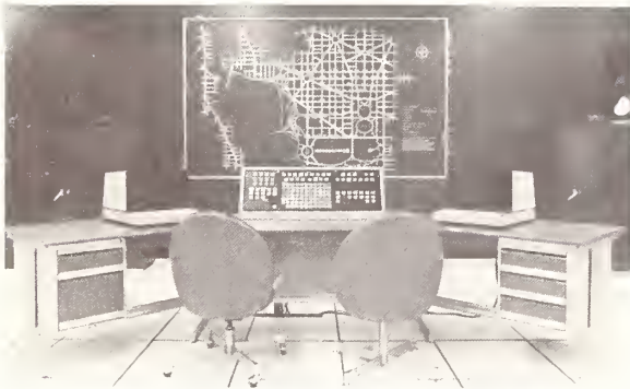
The control center set up to direct bus movement in Washington, D.C. includes a map mechanism that pinpoints participating buses' locations.
