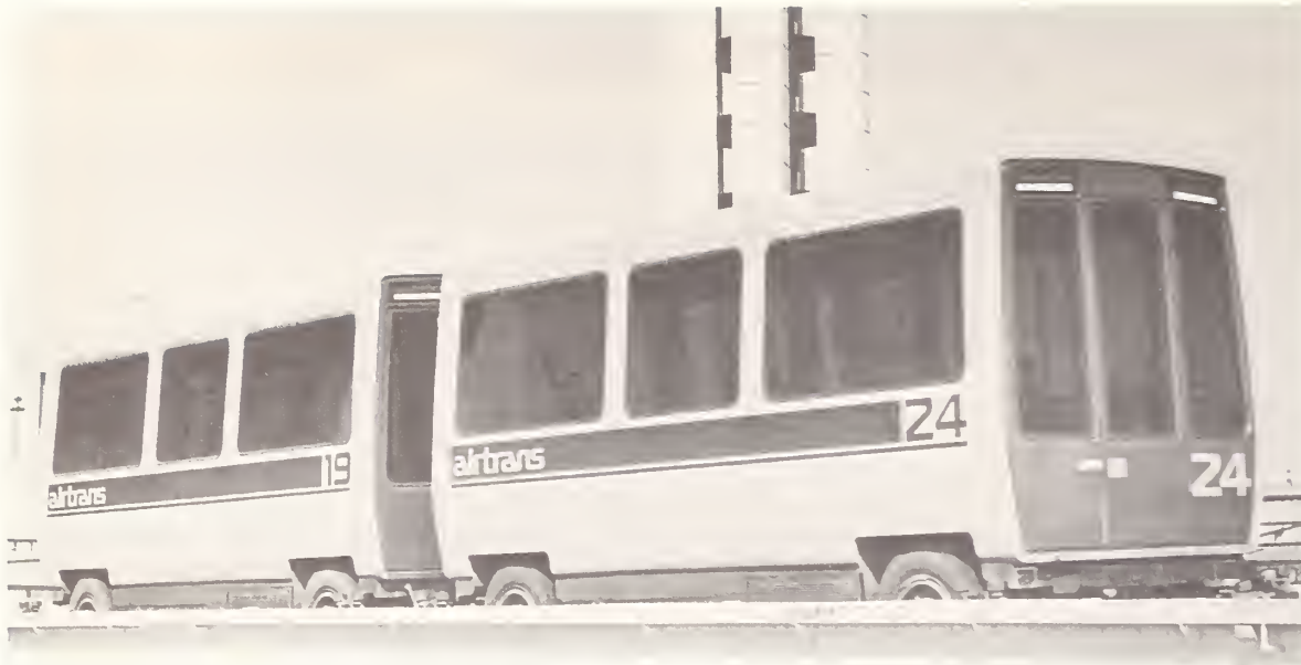
AIRTRANS, an automated guideway system at the Dallas/Ft. Worth Airport, carries both passengers and cargo between distant terminals.
