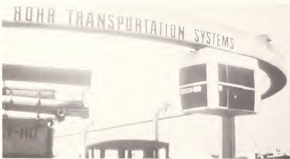
The Rohr Monocab system uses a suspended monorail and electromagnetic propulsion.
