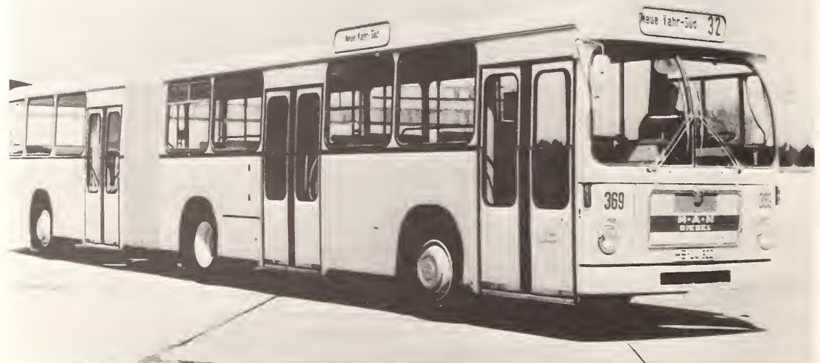
This German-made M.A.N. articulated bus is one form of high capacity vehicle studied for potential U.S. use.
