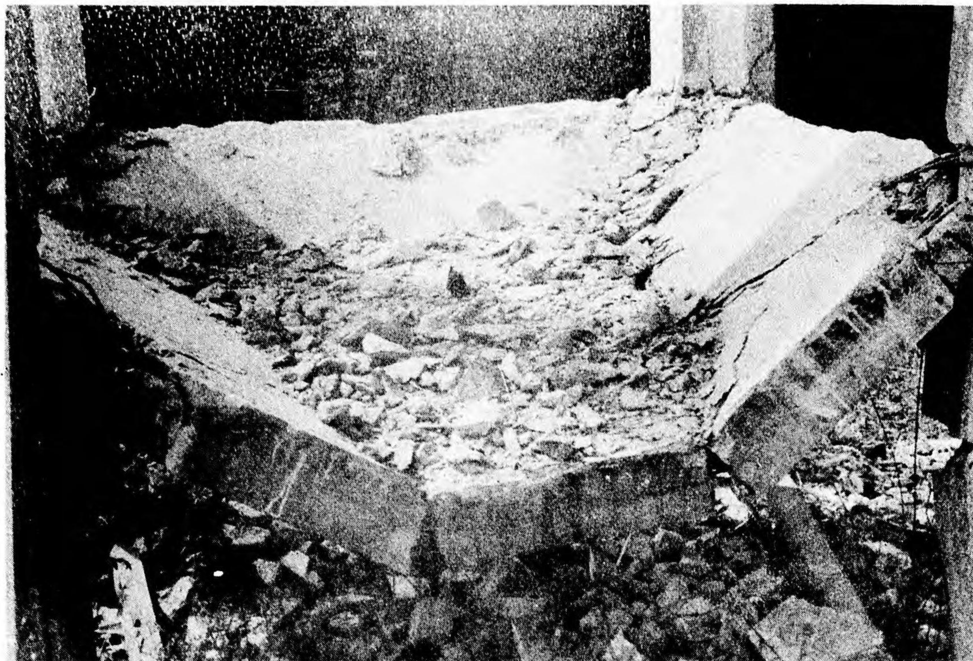
Fig. 11. Upper side of first floor looking down, after detonation of \frac{1}{2} lb of TNT.
