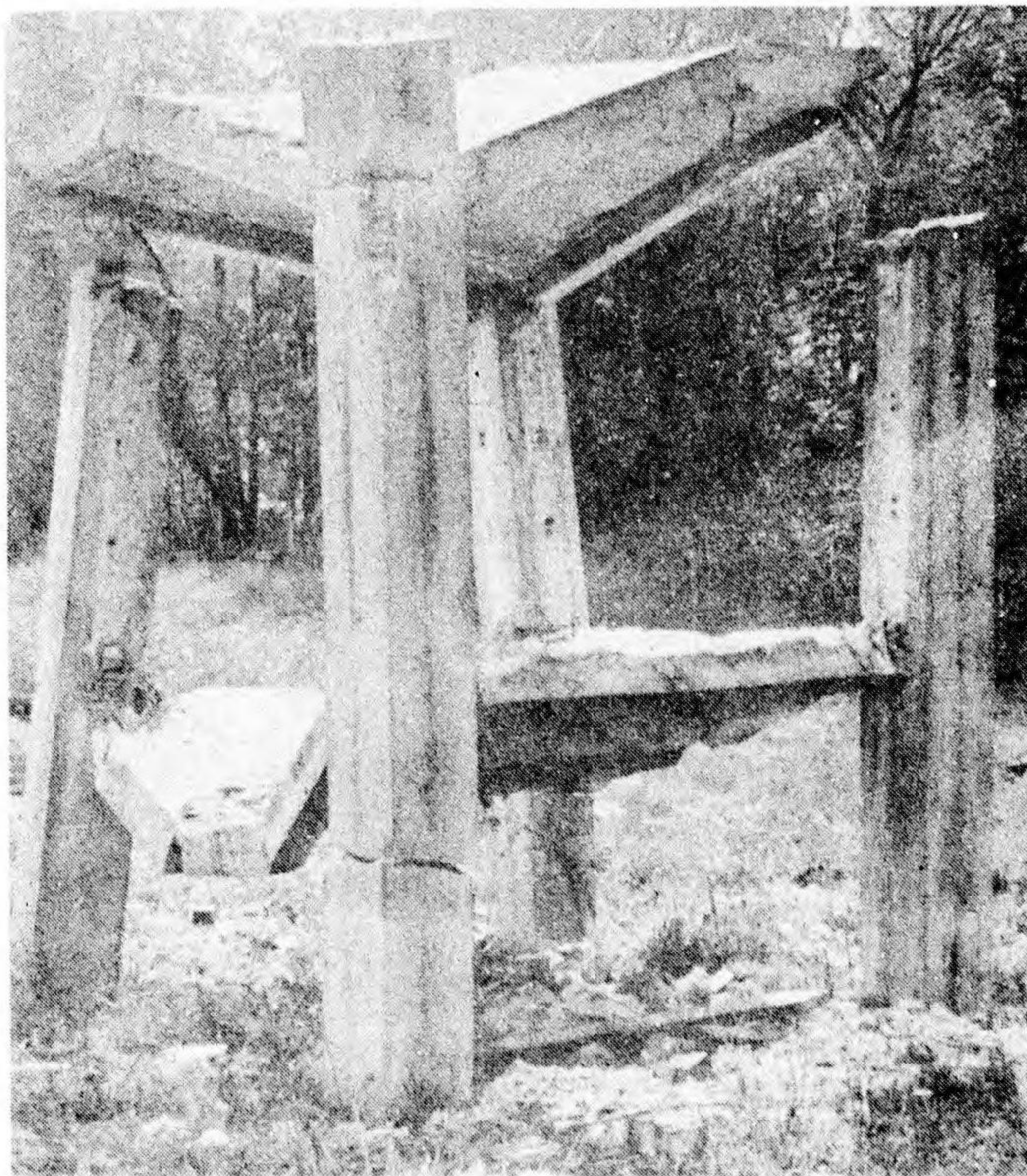
Fig. 8. Test structure viewed from the NW after detonation of \frac{1}{2} lb of TNT.
