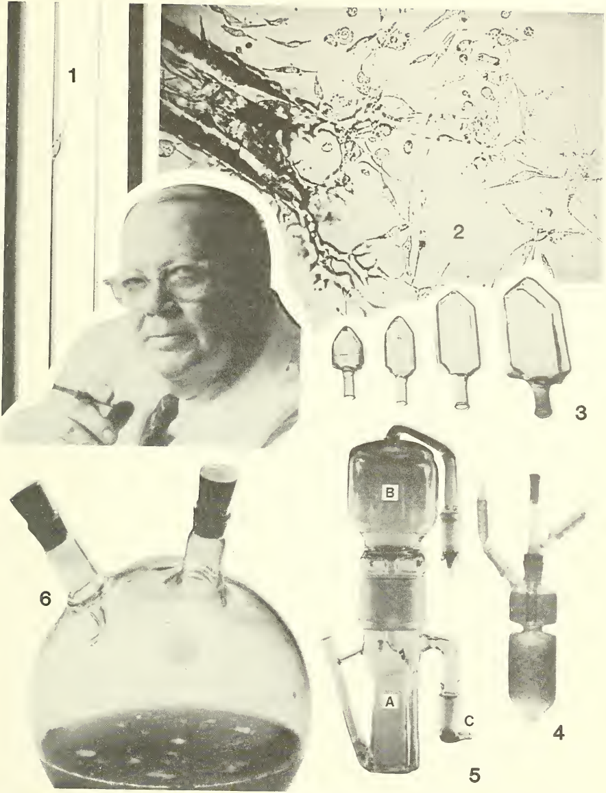
WILTON EARLE and cell culture vessels. 1. Tissue cell isolated in glass capillary tube. 2. Proliferating cells emerging from tube. 3. Pyrex flasks for quantitative growth studies. 4. Three-dimensional substrate culture on glass helices in aerated medium. 5. Substrate culture on multifolded perforated cellophane sheet in medium intermittently forced from A to B by CO 2 in air through C. 6. Shaker flask for propagating multimillion-cell culture in agitated fluid suspension.
