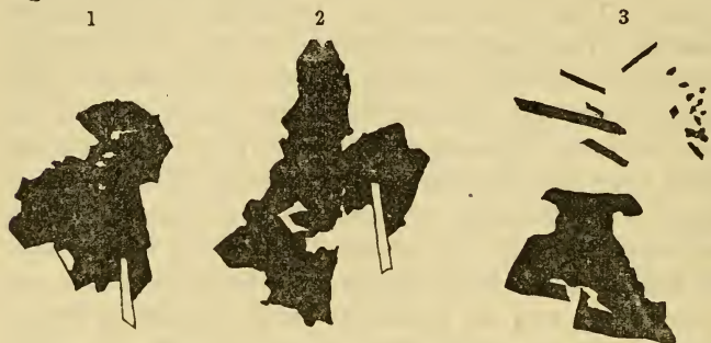
Figures 1 and 2.—Grains of magnetite penetrated by blades of feldspar. ( \times 78 .)
