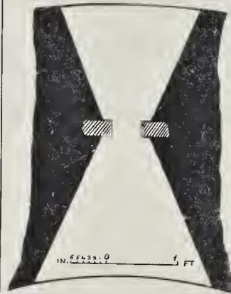
Fig. 3.—Double-splayed Light in the West Front of Trier.
