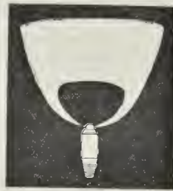
Fig. 21.—Slit Union Burner and Flame.
