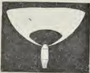
Fig. 18.—Batswing Burner and Flame.
