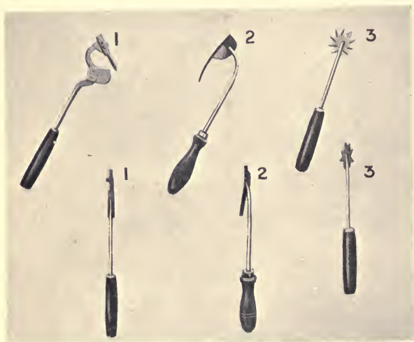
FIG. 7.—The “Bowman-Northway” Tapping Implements.
