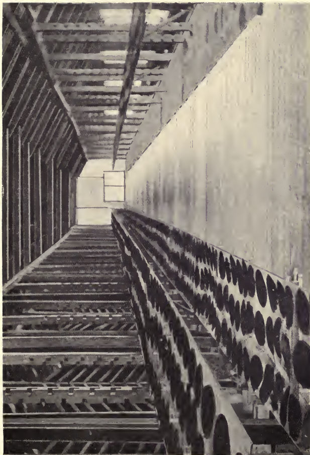
FIG. 17.—Para Rubber "Biscuits" being dried in a Tea-leaf Withering House, Ceylon. (From a photograph by the Author.)
