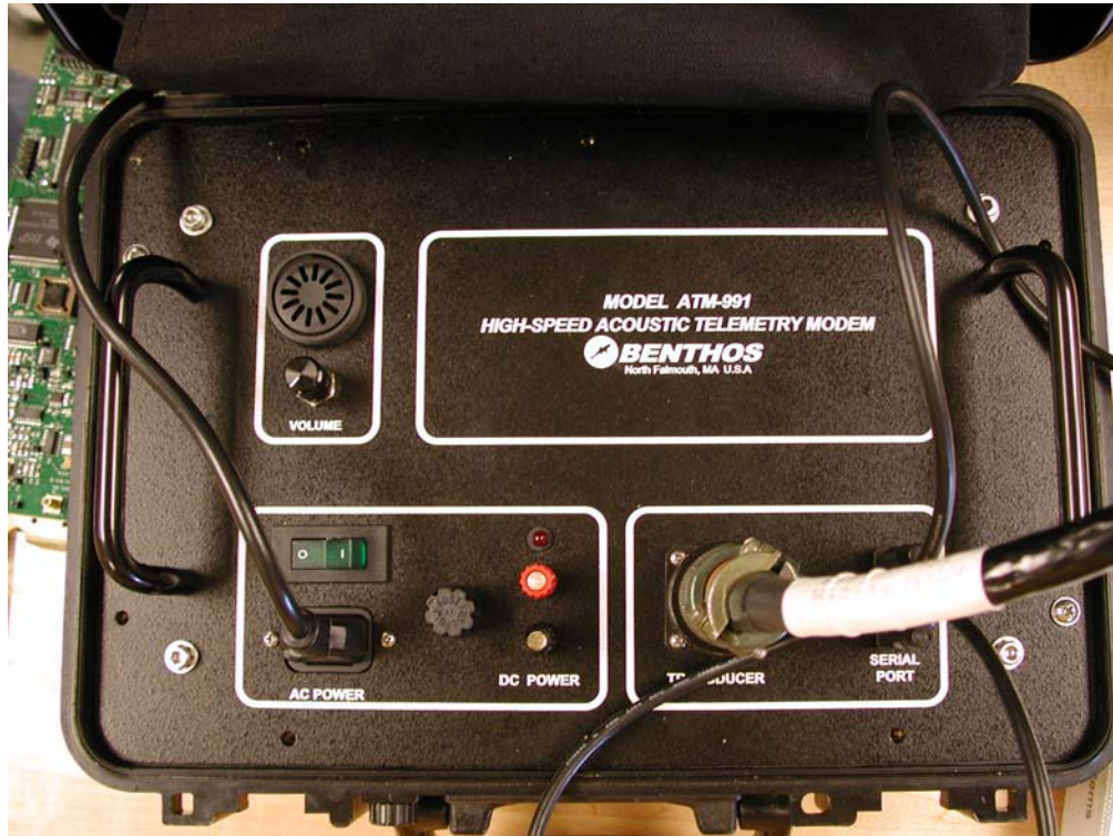
Figure 50. Benthos Deck Box Modem
