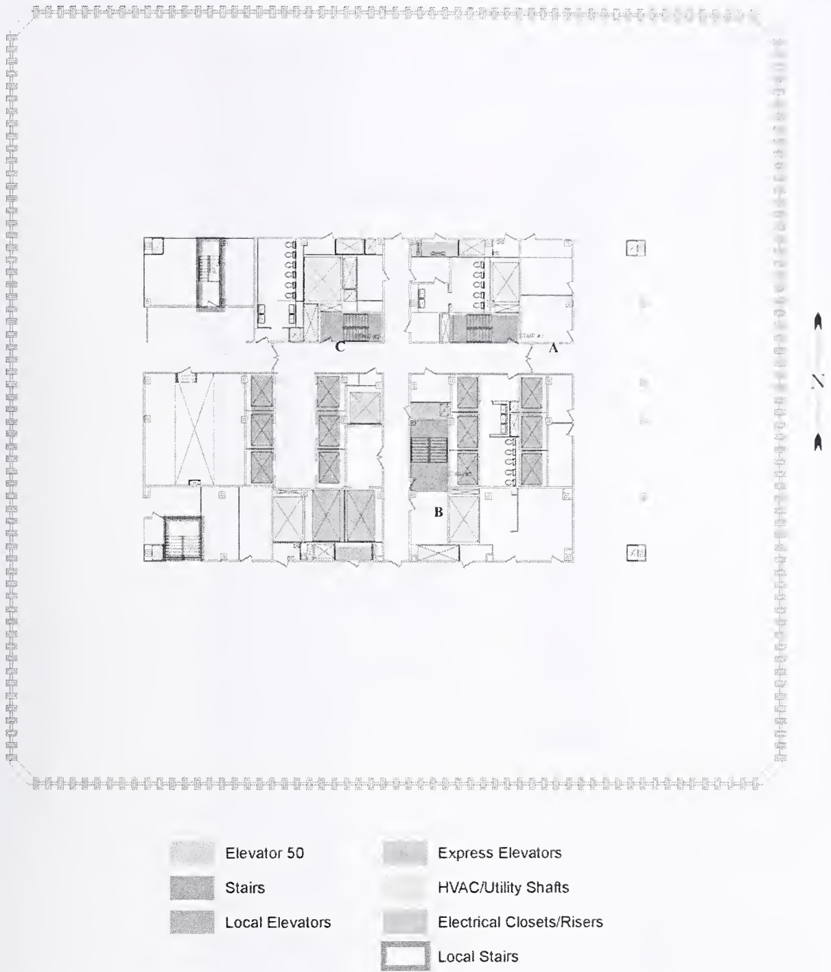
Figure 5–2. Floor layout, 95th floor, WTC 1, North Tower.
